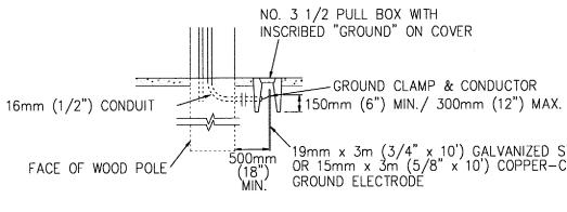
INSTALLATION SHOWN IS FOR SIDEWALK OR PAVED AREAS. IN UNPAVED AREAS, TOP OF BOX SHALL BE RAISED 25mm (1") ABOVE GROUND.
