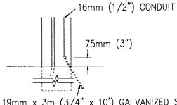
19mm x 3m (3/4" x 10') GALVANIZED STEEL OR 15mm x 3m (5/8" x 10') COPPER-CLAD GROUND ELECTRODE
