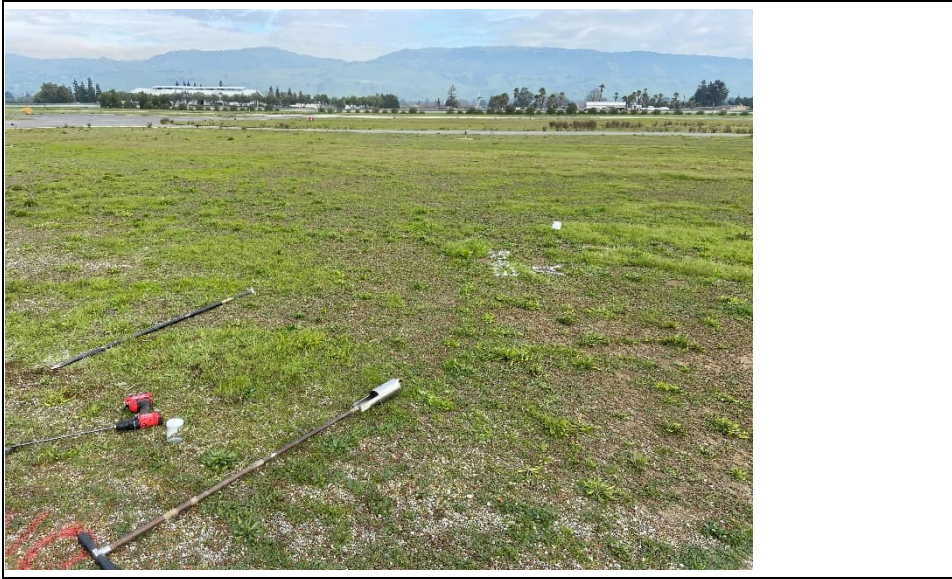
1/17/2022. E16-05: Sampling point relocated 13 feet towards taxiway due to significant gravel.
