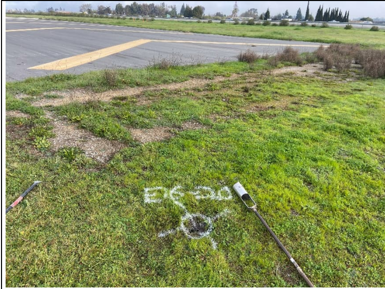
1/18/2022. E16-20: Sampling point relocated 13 feet from original point (pre-excavation).
