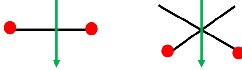
Figure B-7. Example Scenario 2 Configurations. Black lines represent runways, green arrows represent wind direction, and red dots represent the runway-end identified as active
