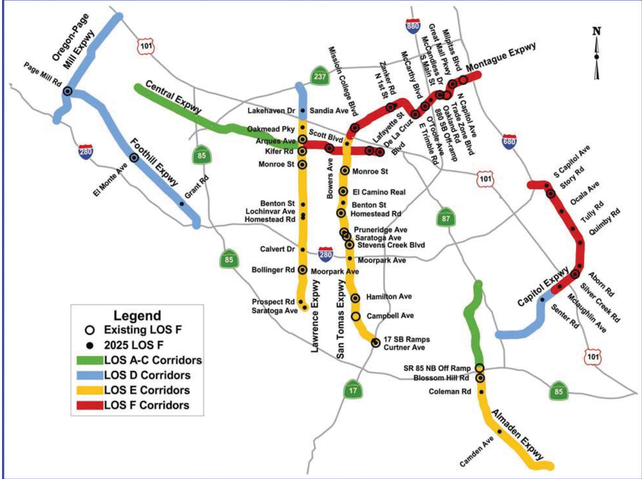
Figure 3-2a: Corridor Level of Service for No Project
