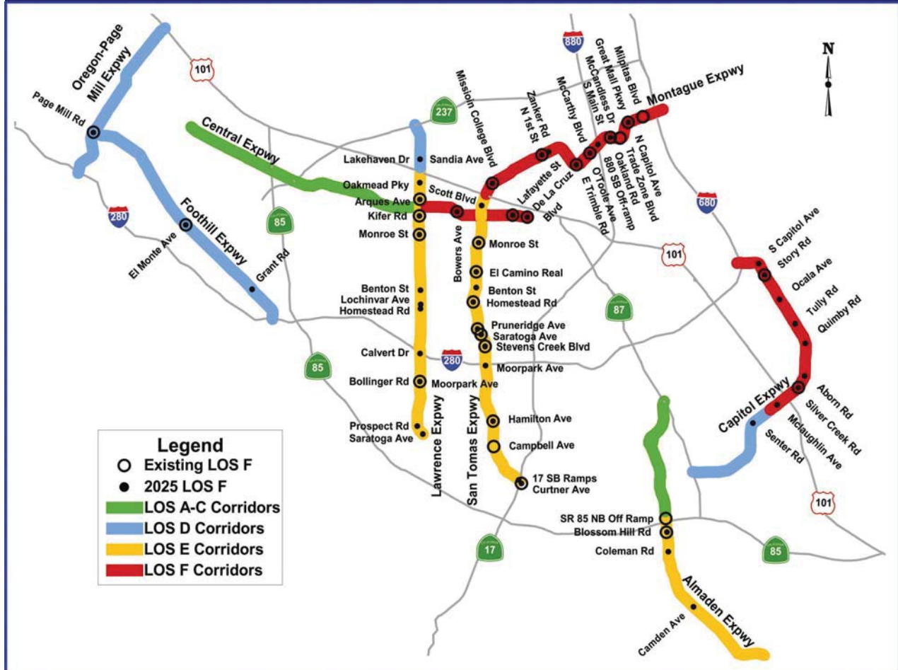
Figure ES-2: Corridor Level of Service for No Project
